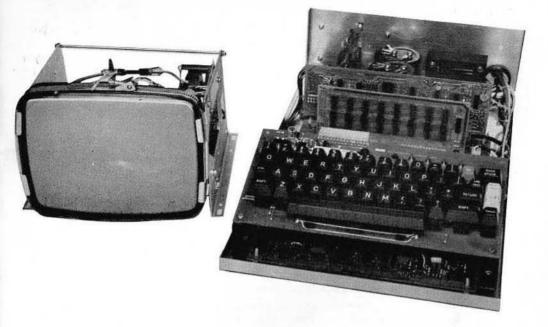
The CT-64 Terminal System kit is a low cost, ASCII stand alone computer terminal for use with either resident or remote computer systems. The display format of the CT-64 is 32 or 64 characters/line, 16 lines per page, 2 pages of storage and either page or scrolling operation with upper and lower case characters.
